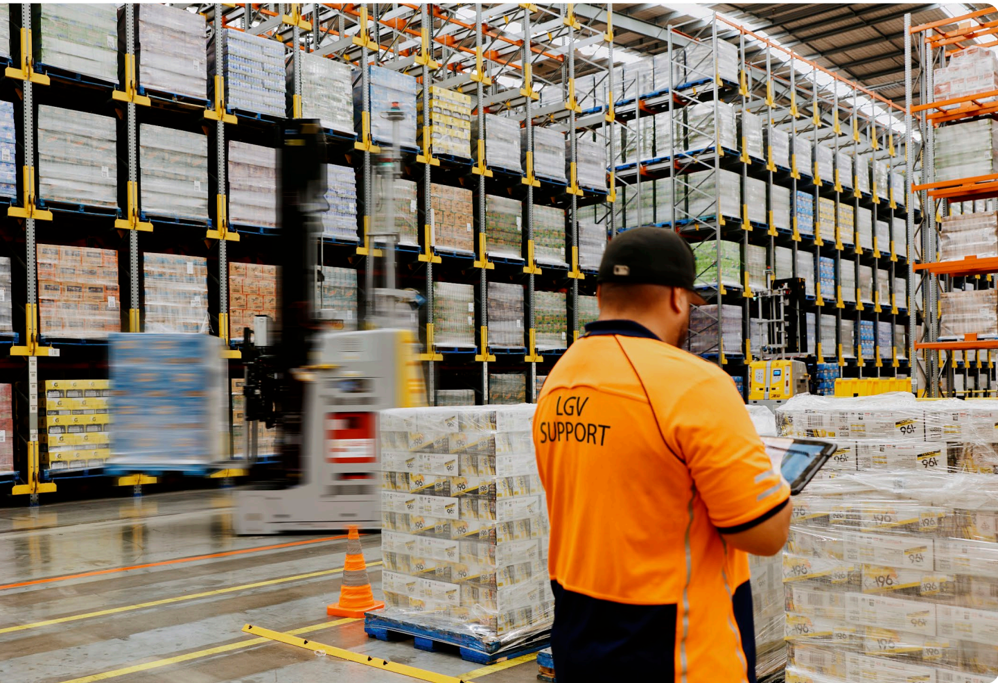
Suntory Oceania’s ‘The Vault’ facility uses laser-guided vehicles (LGVs) to collect pallets of product and move them to trucks for delivery.
