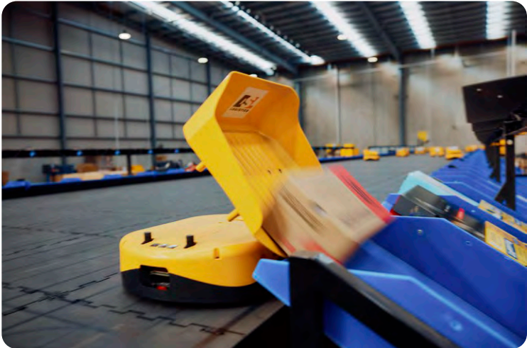
DSL robots scan, sort, and route items, while team members oversee the robots and manage the sorting operations.
